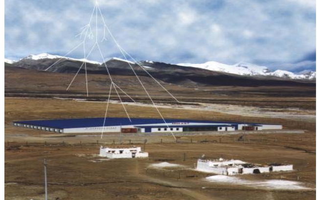
The Yangbajing High Altitude Cosmic Ray Laboratory (4,300 m.a.s.l.) showing the ARGO-YBJ detector, an air shower detector array covering an area of about 6,700 square metres in Tibet. (Credit: INFN / ASPERA)
