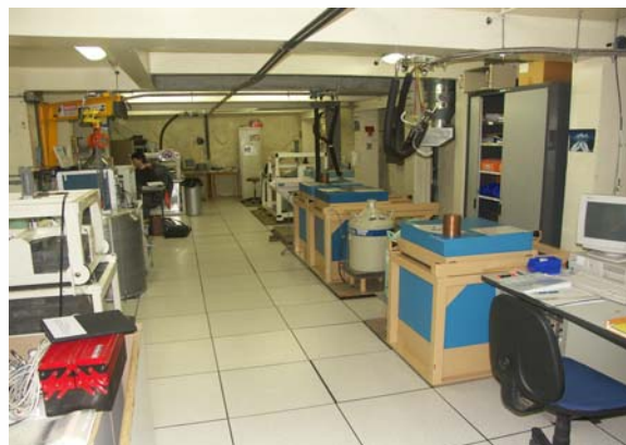
Gamma spectrometers protected by lead shielding at Modane Underground Laboratory (Credit: LSM)
