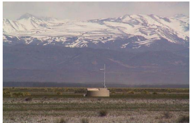
The Pierre Auger observatory consists of 1,660 detectors distributed on a 3,000 square kilometres area in Argentina (Credit: Pierre Auger collaboration / ASPERA).
