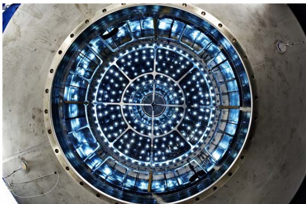
Fisheye view inside the 3-m CLOUD chamber through the lower manhole showing the UV fibre optic illumination and transparent HV electrodes (Credit: Maximilien Brice, CERN )
