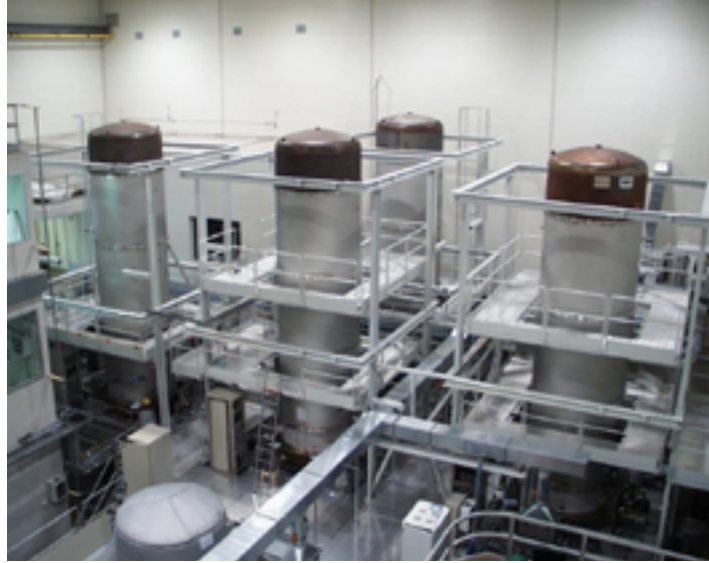
Figure 3 - The Virgo towers; 11 m high, 2.0 m diameter.
