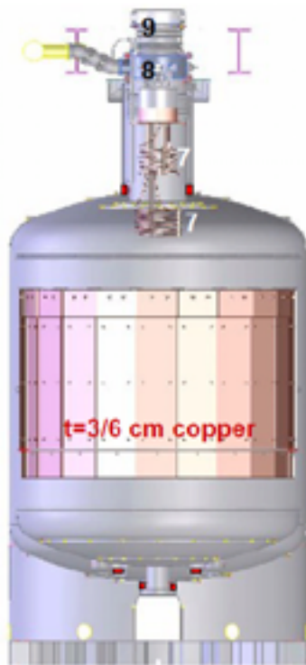
Figure 2 - Characteristics of the GERDA cryostat, and its cross section with active cooling system (7), manifold (8) and the interface (9) to the lock consisting of a bellow and a DN630 shutter. The tiny red rectangles show the locations of the Torlon support and alignment pads of the inner vessel. The bellow in the neck of the inner vessel for compensating thermal shrinkage is barely visible. Detailed drawings are available at [5].
