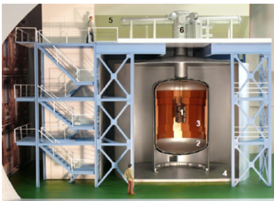
Figure 1 - Model view of the GERDA experiment in Hall A of LNGS showing the germanium detector array (1), the LAr cryostat (2) with the internal copper shield (3), the surrounding water tank (4), the clean room (5) and the lock (6) through which the Ge detectors are deployed into the cryostat. For clarity, the detector array is enlarged.
