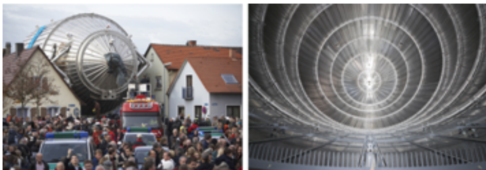
Figure 3 - Left: arrival of the large main spectrometer vessel at KIT after an 8800 km journey. Right: wire electrodes on the inner wall of the main spectrometer, which was installed under cleanroom conditions.
