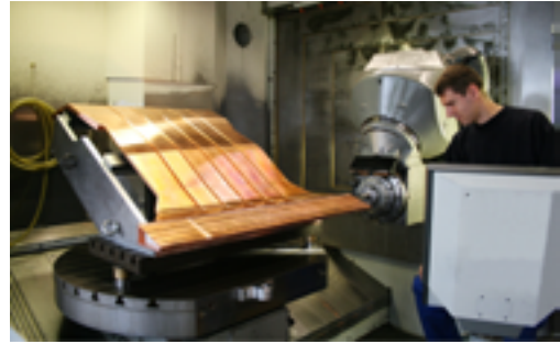
High heat loaded components for JET
