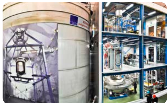
XENON1T installation in the underground hall of Laboratori Nazionali del Gran Sasso (Credit: Roberto Corrieri and Patrick De Perio)
