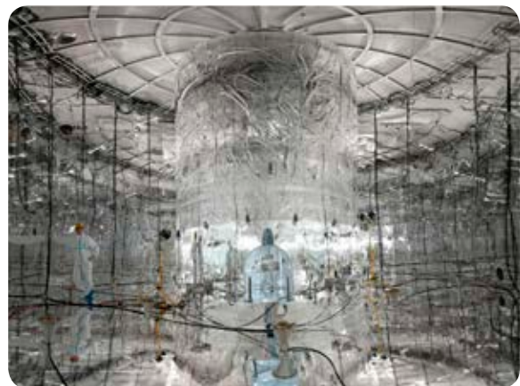
The inner walls of the water tank are covered by a reflecting foil improving the light detection. This permits the identification of cosmic muons. © K. Freund, GERDA collaboration
