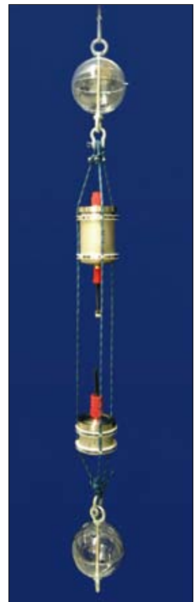
Setup to test the feasibility of acoustic detection of neutrinos in ice.
