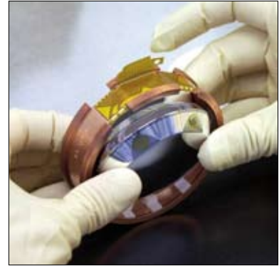
High-purity germanium crystals for dark matter search.
