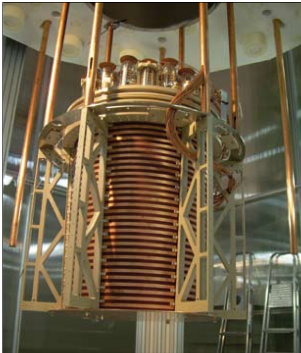
The central part of a 100-litre liquid argon detector being installed by the WARP collaboration in the Gran Sasso Laboratory.
